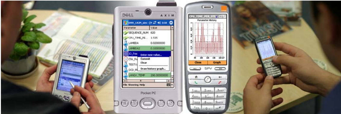
Figure 4. The PDA and Smartphone Clients provide a mobile user interface for monitoring and tweaking (steering) simulation parameters in real-time (left), additionally incorporating visual parameter value trend plotting capabilities (right) to aid understanding of how experiments change and evolve as they run.
