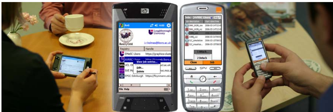
Figure 3. The RealityGrid PDA and Smartphone Clients both provide a mobile facility to query a Registry (left) and retrieve a list of currently deployed jobs (right). Once a job has been selected, each Client will then attach (connect) remotely to the appropriate scientific application running either on or off the Grid.
