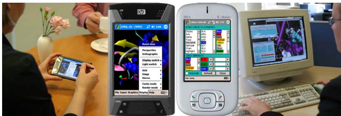
Figure 6. When using the RealityGrid PDA or Smartphone Clients (left), researchers who employ VMD [13] on a daily basis are able to access and interact (through their handheld device) with familiar, indigenous user interface facilities from their everyday desktop or workstation application (right).
