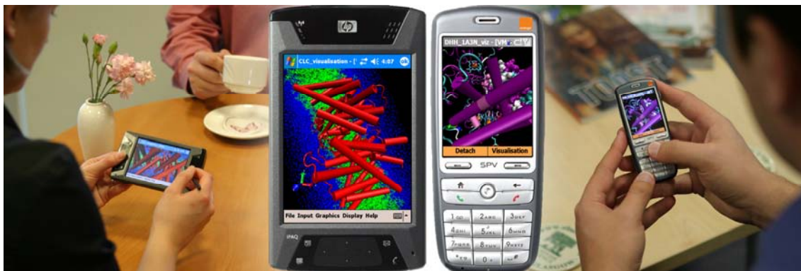
Figure 5. The handheld RealityGrid Clients each offer the researcher an inclusive provision of advanced, visualisation-oriented interaction facilities, which (up until this point) would only typically otherwise have been accessible through conventional desktop (or laptop)-based user interface applications.
